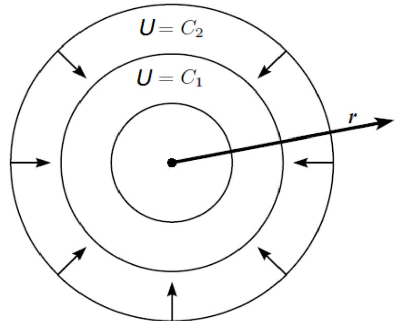
**Gradient** – example (field of positive electrical charge): (2/3)
