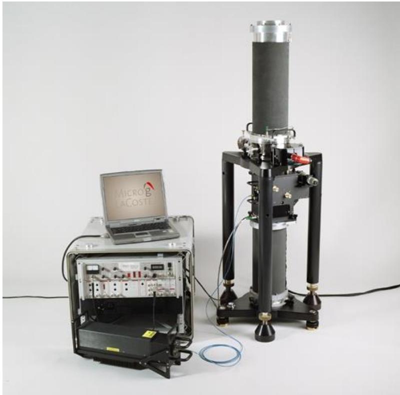
free-fall instrument (absolute gravimeter)
