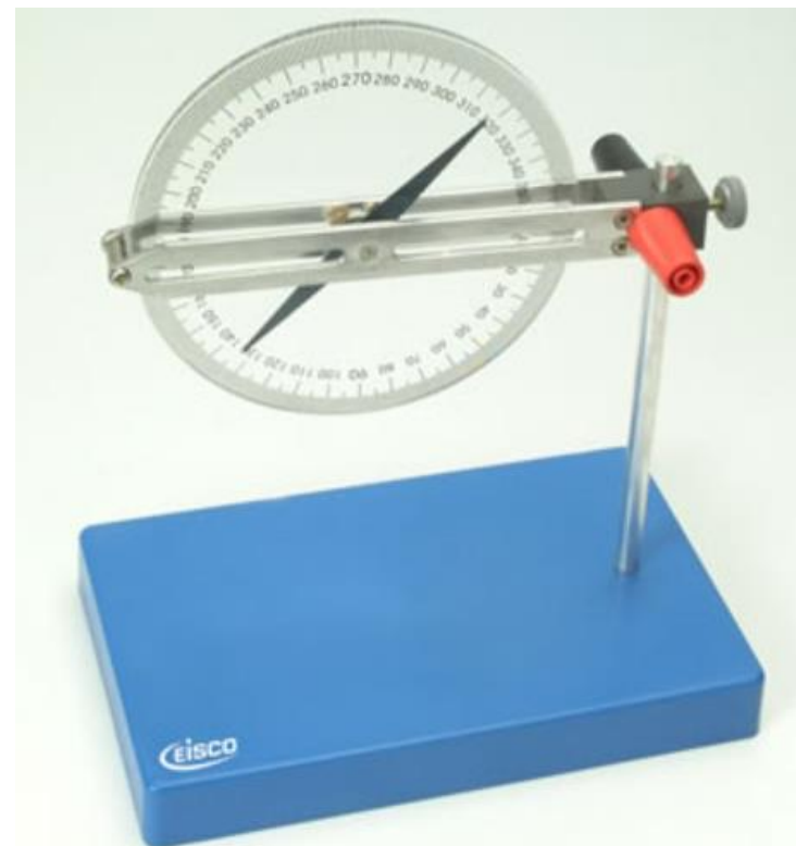
PH0832N Magnetic Needle Inclination/Declination Demonstration Compass
