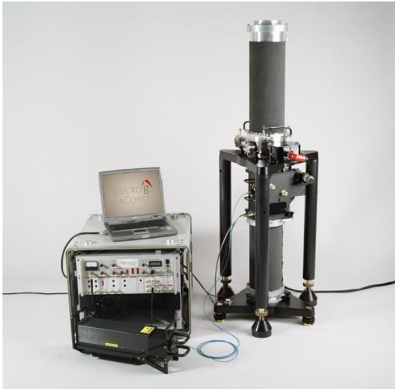
free-fall instrument (absolute gravimeter)
