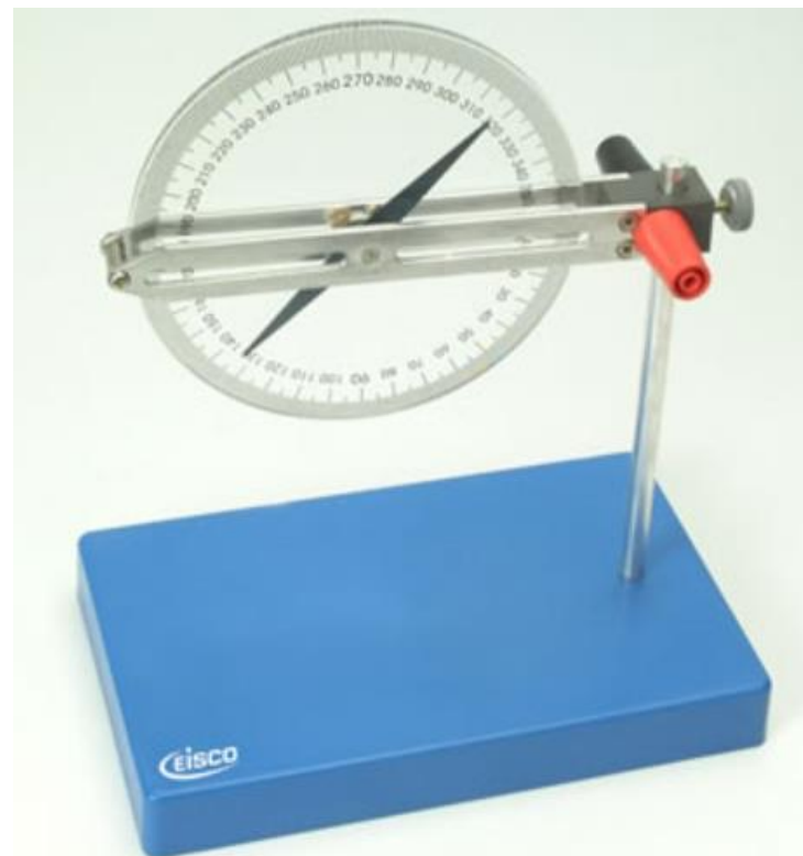
PH0832N Magnetic Needle Inclination/Declination Demonstration Compass
