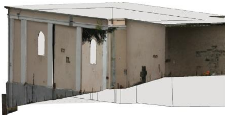
FIGURE 6 Digital model of the church without a roof displayed with original textures in PhotoModeler Scanner software.
